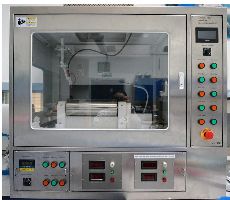
Figure 3.2. Electrostatic spinning device.
