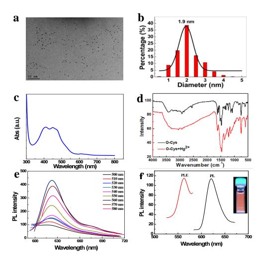
Fig. 1. (a) TEM images of O-Cys. (b) Corresponding size distribution of O-Cys. (c) Normalized UV-vis absorption of O-Cys. (d) The FT-IR spectrum of O-Cys, mixed solution of O-Cys and  $Hg^{2+}$ . (e) PL spectrum of the O-Cys at different excitation wavelengths from 500 to 580 nm; both the excitation and emission slit widths were 5 nm. (f) Fluorescence excitation spectra and emission spectra of O-Cys aqueous solution at room temperature (25°C). Inset: photographs of O-Cys aqueous solution.
