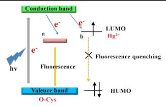
**Scheme 2.** Schematic for the fluorescence quenching mechanism according to molecular orbital theory in the absence (a) and presence (b) of Hg<sup>2+</sup>.
