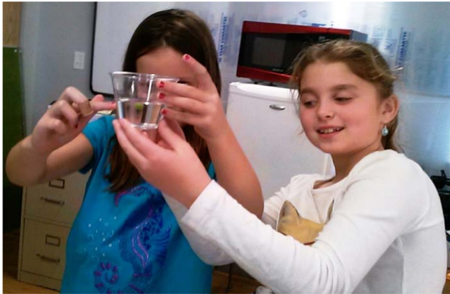
Figure 9. Pea becomes buoyant in 90 mL of water after dissolving 5 level teaspoons of sugar.
