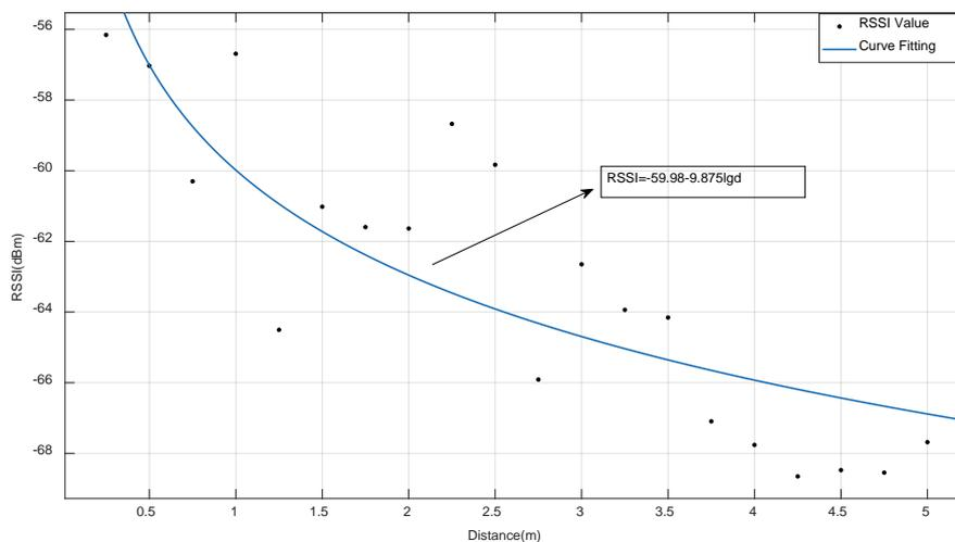
Figure 4. Fitting curve diagram after combined filtering within 1~5m
