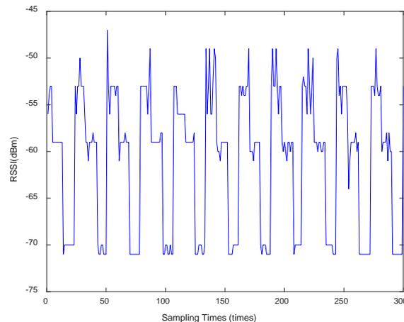
**Figure 1.** Fluctuation diagram of RSSI signal received at a distance of 1m
