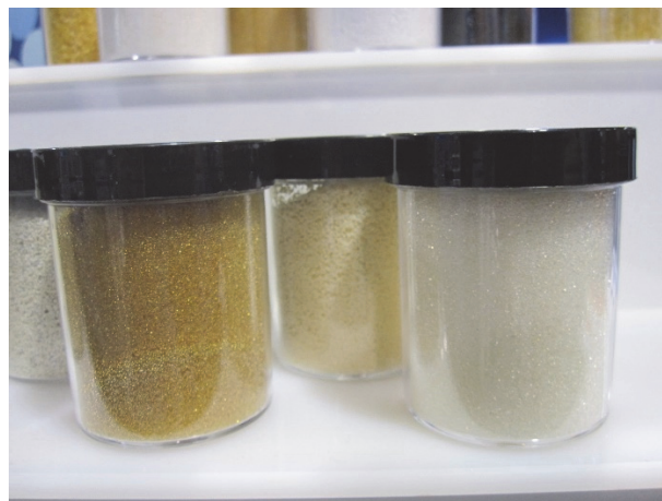
Figure 9. What ion exchange media should look like
