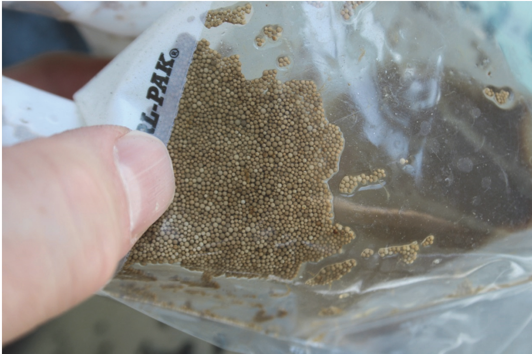
Figure 8. Poisoned Ion exchange media
