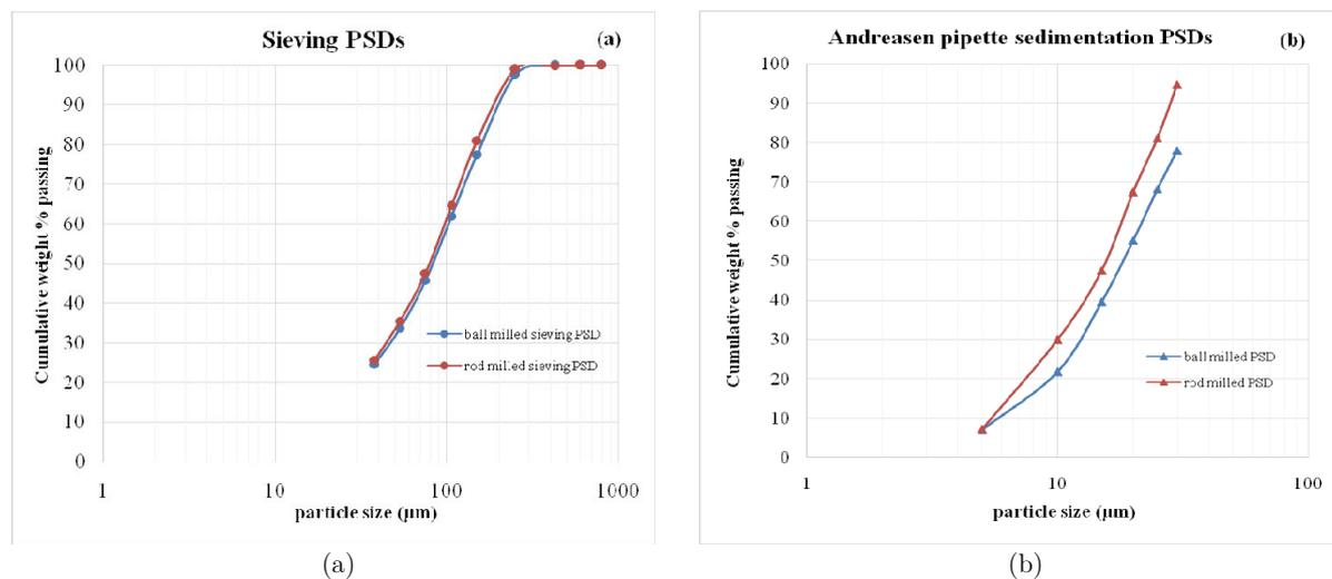
**Figure 3.** PSDs of quartz minerals ground in ball and rod mill by (a) Sieving and (b) Andreasen pipette sedimentation techniques (Redrawn from [21])
