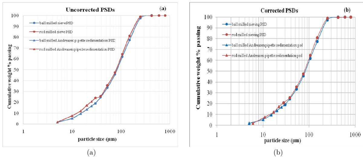
**Figure 4.** (a) Uncorrected and (b) Corrected PSDs of ball and rod milled quartz by combination of PSDs measured by sieving and Andreason pipette sedimentation techniques (Redrawn from [21])
