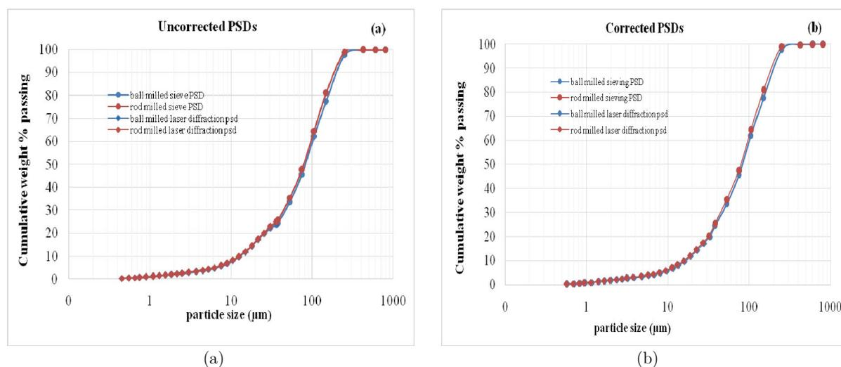
**Figure 7.** (a) Uncorrected and (b) Corrected PSDs of ball and rod milled quartz by combination of PSDs measured by sieving and laser diffraction techniques (Redrawn from [22])
