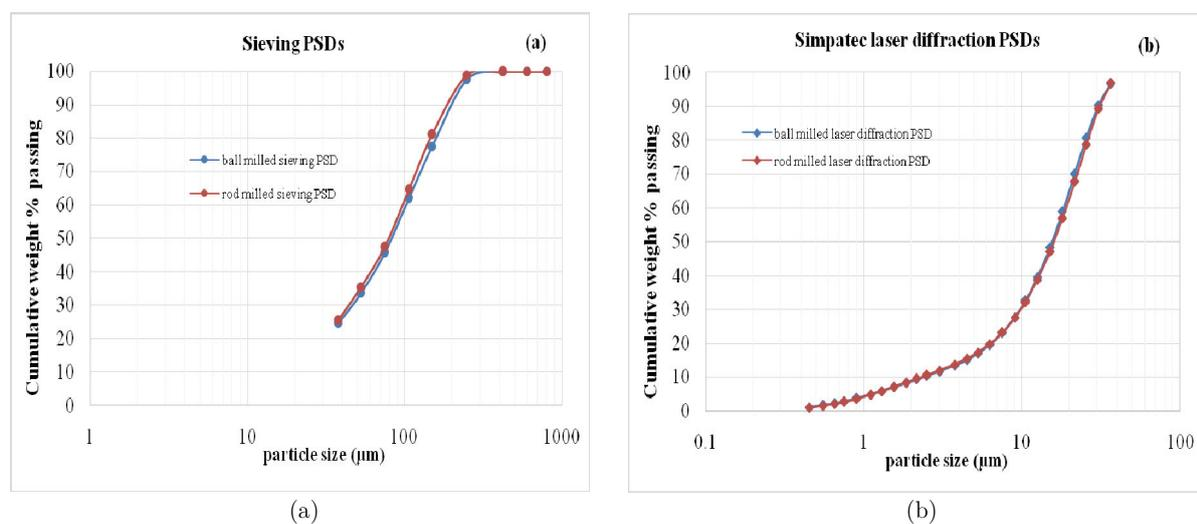
**Figure 6.** PSDs of quartz minerals ground in ball and rod mill by (a) Sieving and (b) laser diffraction techniques (Redrawn from [22])
