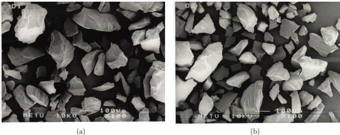
**Figure 5.** SEM microphotographs for (a) ball and (b) rod mill products of quartz (x100) (from [21, 22])
