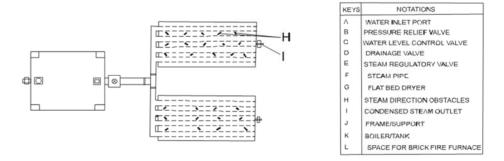
Figure 3. Orthographic plan view of the developed platform with steam heat exchangers for drying of parboiled paddy rice and other agricultural products
