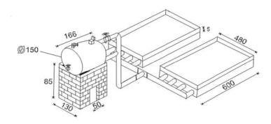
Figure 1. Isometric view of the developed platform with steam heat exchangers for drying of parboiled paddy rice and other agricultural products (All dimensions are in mm)
